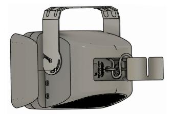
The default setting of the speaker is optimally adjusted for use with Wet Sounds Venue Series Amplifier (40hm). In the instance of using the speakers with a 70v distributed load amplifier, remove 2x Phillips head screws and tap adjustment cover. Adjust the rear tap to the desired wattage that satisfies your system requirements and reinstall the cover.
