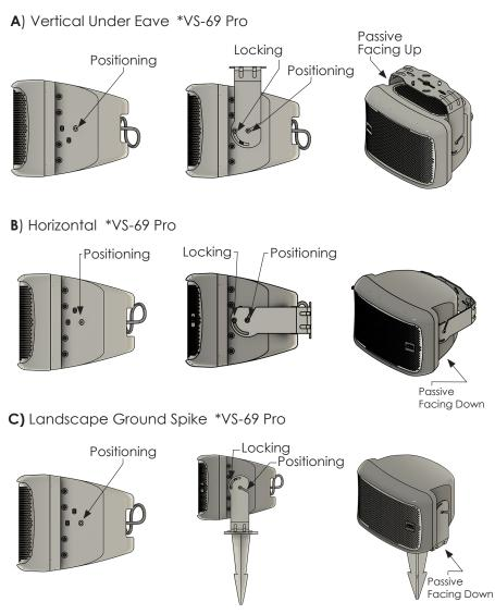
\*If using optional Ground Spike, securely mount the bracket to ground spike, place spike in desired landscape location and follow speaker mounting instructions above.
