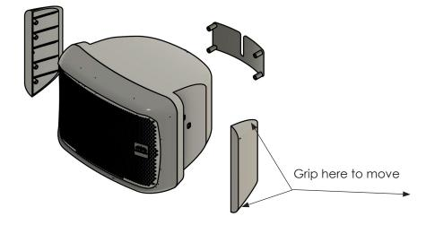
**Step 2** - Pre-thread hardware in the speaker positioning locations based on desired mounting orientation shown below.
