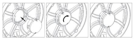
The above diagram shows the installation of the tweeter. Insert & rotate the tweeter clockwise. The removal of the tweeter is the opposite.
