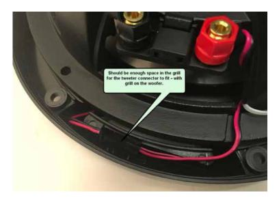
**4.** With the grill in place, route the RGB LED wire through the slot in the basket & make sure the RGB wire is flat against the lip of the basket. Affix the RGB wire into the slot using a wire tie.
