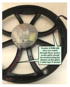
**2.** The tweeter wire on the woofer should be routed through the opening in the basket. The RGB wire has a separate opening in the basket.
