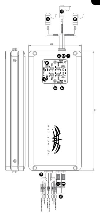
**NOTE** - When using the **STX-MICRO 4** in **Bridged Mode**, the 2CH/4CH Switch should be in the 2CH position.
